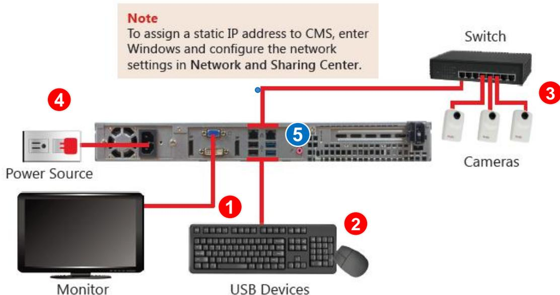
1. Connect the VGA monitor using the VGA cable supplied by the monitor manufacturer.
