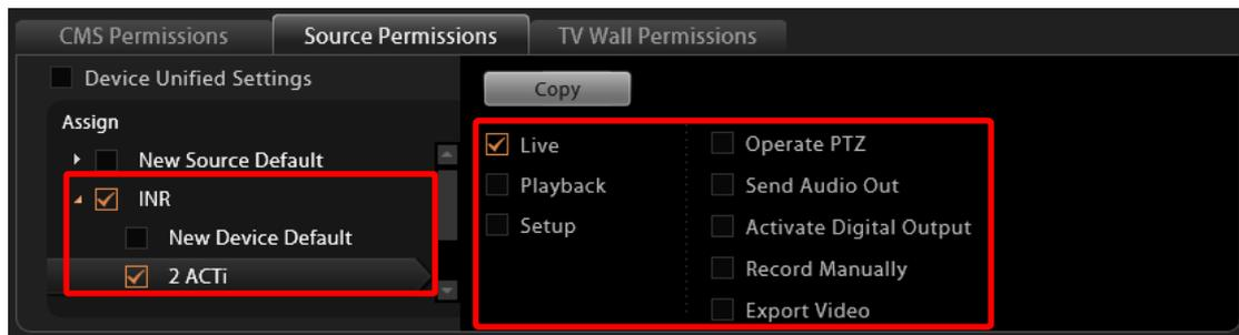
Instead of tailoring the settings for each device, you may click “**Device Unified Settings**” and set universal settings, which will be applied to any device you check under this NVR.
