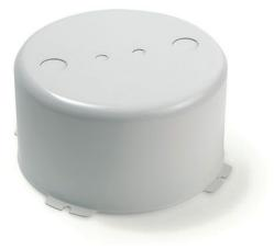
During a fire, the ceiling cavity in which loudspeakers are installed can allow flames to spread throughout a building. To prevent fire entering the cavity via the loudspeaker, the ceiling loudspeaker can be fitted with a steel fire dome. This optional fire dome is mounted on the loudspeaker assembly using four self-tapping screws supplied with the fire dome. The fire dome has knockout holes for two grommets (supplied) and two cable glands (PG 13)
