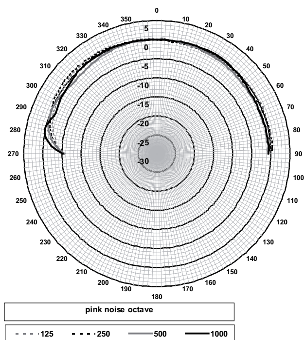
LC3-UC06 horizontal/vertical polar diagram (low frequency). Normalized at 0-degrees axis.
