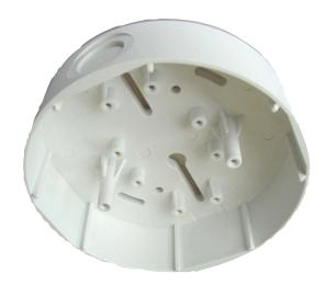
The Additional Base MSC 420 was conceived specially for surface-mounted cable feeds with cable protection conduits and has 2 opposing pre-cut inlets of 20 mm diameter and 2 additional opposing and prepared inlets for up to 28 mm diameter.
