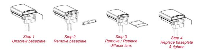
The illuminator is delivered with a 35° beam angle. To alter to 10°, remove the baseplate from the bottom of the product and remove the existing lens and then reattach the baseplate securely. With no lens insert the product produces a 10° beam angle.
