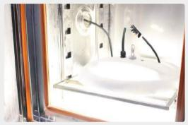
The test equipment opening 2hours, keeping temperature<-40°C, the lamp working fine. The test equipment opening 4hours, keeping temperature>60°C, the lamp keep working fine.
