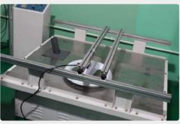
Vibration test is a simulation of various vibration condition including transportation, installation and using, to ensure system robustness.
