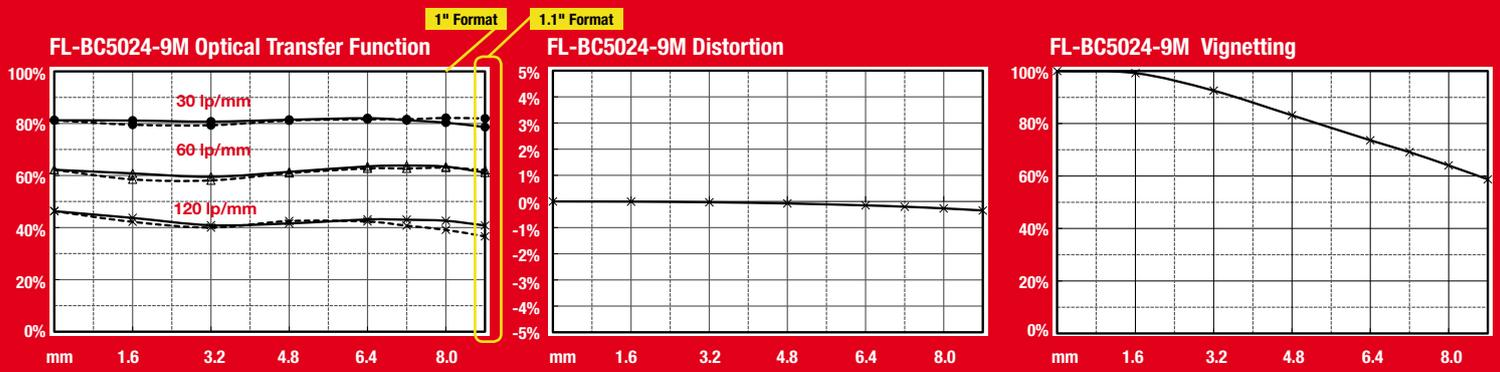
Supports 1" format, 9 megapixel / 1.1" format 12 megapixel cameras. Achieves 147 lp/mm high resolution from centre to the periphery. The lenses are not only optimised for high image quality, but also for use in harsh environments and durable industrial systems.
