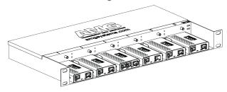
3. Fix the rack chassis into the 19inch rack using 4 screws and cage nuts (not provided) as shown in the image below:
