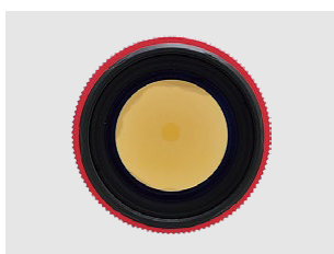
Standard lens showing browning after being subjected to gamma rays.
